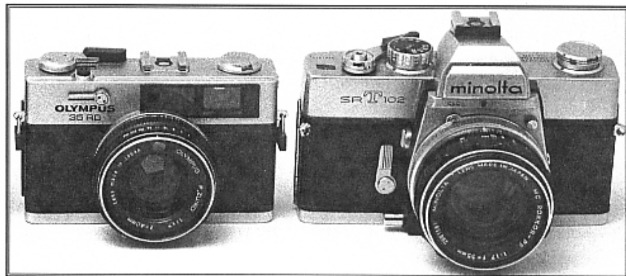
HEAD-TO-HEAD: When it was introduced, the Olympus 35RD matched the features of the top-of-the-line Minolta SRT102 except for the SLR viewing system. But the 35RD came in a much smaller package and had automatic exposure which the SRT cameras lacked.
