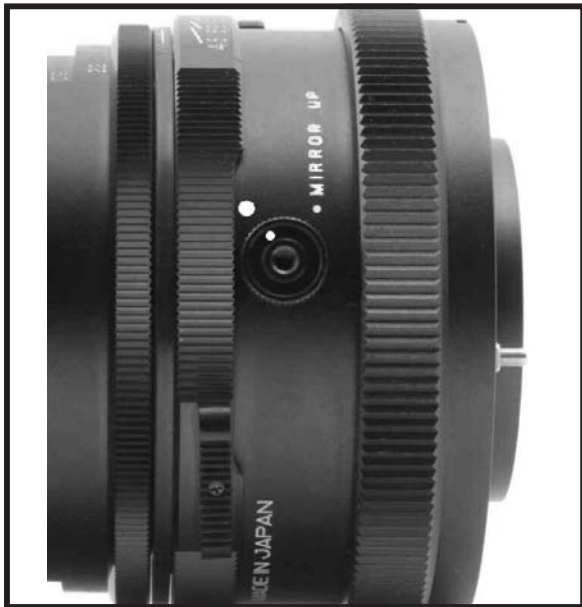
Fig.9 The "Mirror Up" setting closes the shutter without firing it -- but it stays cocked. You release the shutter with a cable release or turning the dial.
