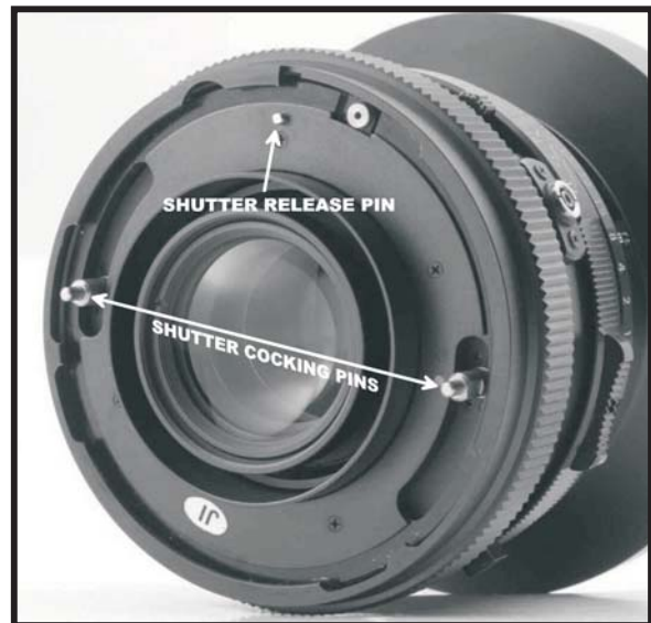
Fig.8 Rear plate of the Mamiya Sekor C 37mm f4.5 Fish-Eye. The rear shutter cocking and releasing pins can easily be used when removed from the camera.
